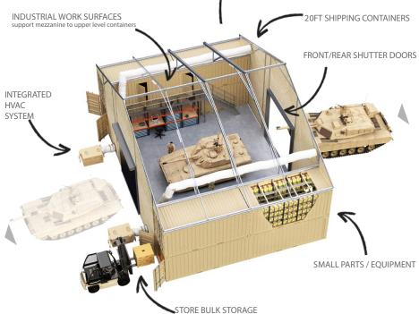
Create a fully functioning containerized maintenance shelter incorporating RACKBOX KITS
